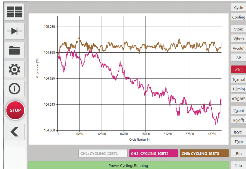
The Simcenter POWERTESTER product displays how the in-cycle junction temperature difference changes during power cycling.
