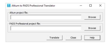
The translator creates a new PADS Layout in the project directory. In this example, it is C:\ALTIUM\_TRANSLATION\ALTIUM\_TO\_PADS\_PRO\USB\_panel\PCB\Board1.pcb
